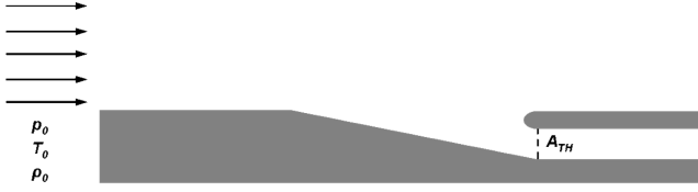
Fig. 6 Schematic representation of a conventional NACA inlet cross section.
